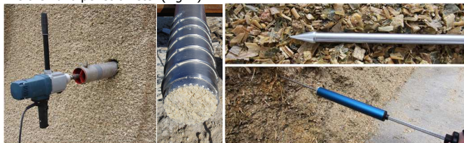
Fig 2. Core sampler (4L volume) and penetrometer to estimate silage density
